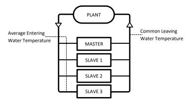
Master performs a so-called Partial control of each Slave unit in the system.
